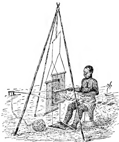
FIG. 37.—Primitive loom with pedals.
